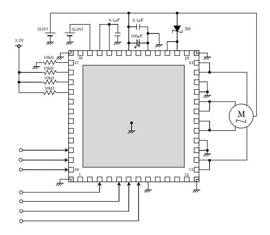
Please mount the four corner pins of the QFN package and the exposed pad to the GND area of the PCB.
