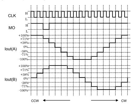
MO output shown in the timing chart is when the MO pin is pulled up.
