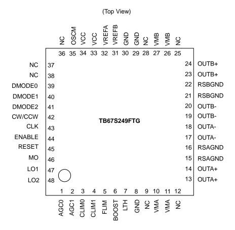
Note: Please solder the corner pad and the rear thermal pad of the QFN package, to the GND pattern of the PCB.
