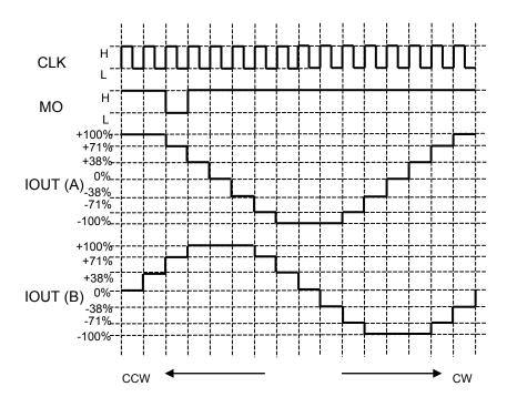
MO output shown in the timing chart is under the condition the MO pin is pulled up.
