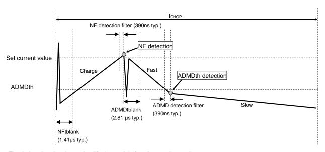
Note: The timing chart has been simplified to explain functions and operations.
