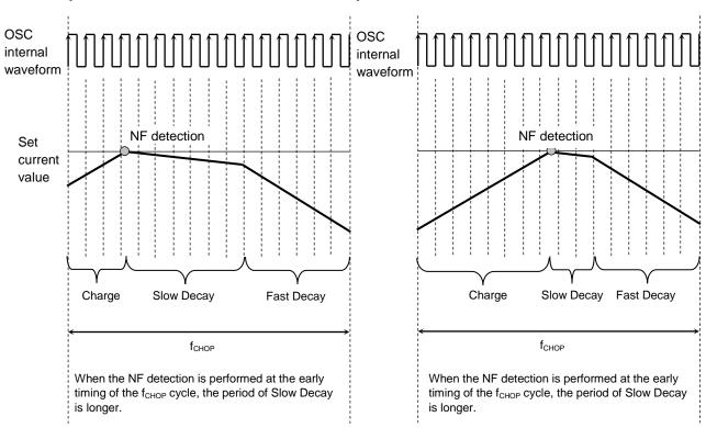
The Charge period (the time required for the current flowing in the motor to reach the set current value) varies depending on drive conditions.
