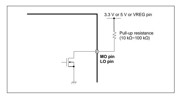
Note: The equivalent circuit diagrams may be simplified for explanatory purposes.
