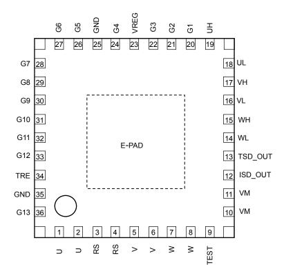
Note 1: Design the pattern in consideration of the heat design because the back side (E-PAD (3.4mm × 3.4mm)) and the four corners of the PAD have the role of heat radiation. (The back side (E-PAD) and the four corners of the PAD should be connected to GND because they are connected to the back of the chip electrically.)
