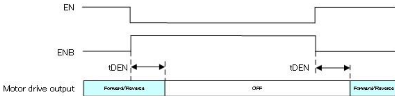
Figure 7.1. EN/ENB signals and motor drive output
