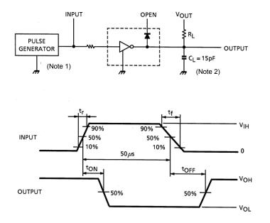
Note 1: Pulse width 50  $\mu$ s, Duty cycle 10%
