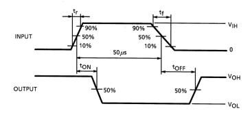
Note 1: Pulse width 50  $\mu$ s, Duty cycle 10% Output impedance 50  $\Omega$ , tr  $\leq$  5 ns, tf  $\leq$  10 ns, V<sub>IH</sub> = 5.0 V
