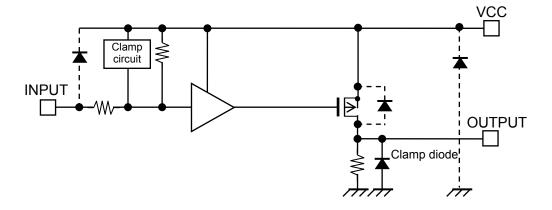
Basic circuit may be omitted partially or simplified for explanatory purpose.
