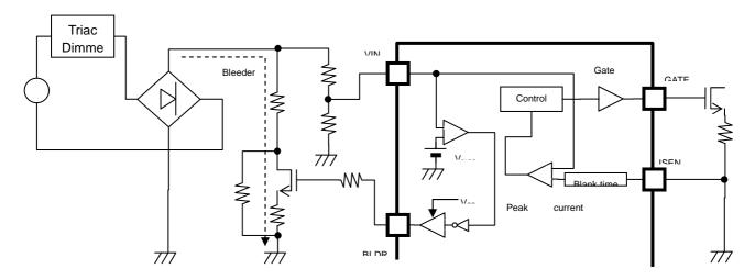
Conduction angle of modulation AC signal of the triac dimmer input to the VIN terminal is detected in threshold  $V_{\text{ANG-DET}}$ . The LED current is changed by adjusting  $V_{\text{PEAK}}$  by the detection result.
