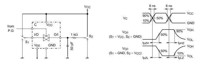
2. Cross Talk (control input-switch output) fIN = 1 MHz duty = 50% tr = tf = 6 ns
