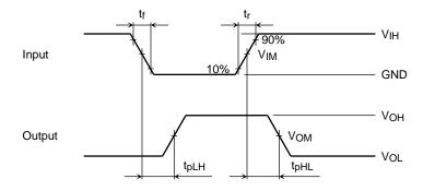
Figure 2 t<sub>pLH</sub>, t<sub>pHL</sub>
