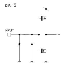
**Bus Terminal Equivalent Circuit**
