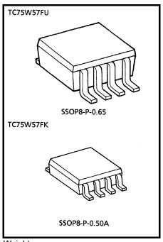
Weight SSOP8-P-0.65: 0.021g (typ.) SSOP8-P-0.50A: 0.01g (typ.)
