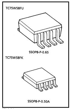
Weight SSOP8-P-0.65: 0.021g (typ.) SSOP8-P-0.50A: 0.01g (typ.)
