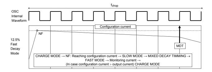
Constant current PWM control mode: Current waveform when configuration current changes by changing Vref
