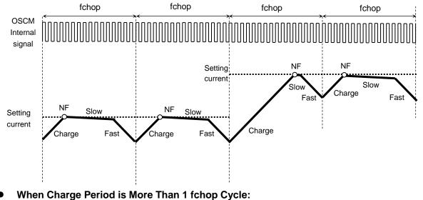
When the Charge period is longer than fchop cycle, the Charge period extends until the motor current reaches the NF threshold. Once the current reaches the next current step, then the sequence goes on to Decay mode.
