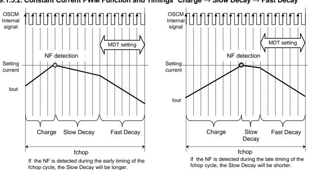
9.1.5.2. Constant Current PWM Function and Timings \*Charge  $\rightarrow$  Slow Decay  $\rightarrow$  Fast Decay
