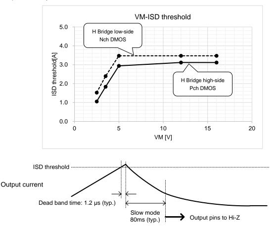
Note: Above ISD operation threshold value and band times are reference values, and are not guaranteed.
