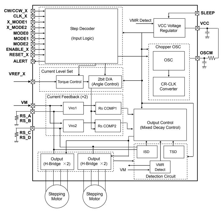
\* "X" means the ellipsis of AB / CD of each Ch. (CW/CCW\_X,CLK\_X,X\_MODE1,X\_MODE2,ENABLE\_X,RESET\_X)
