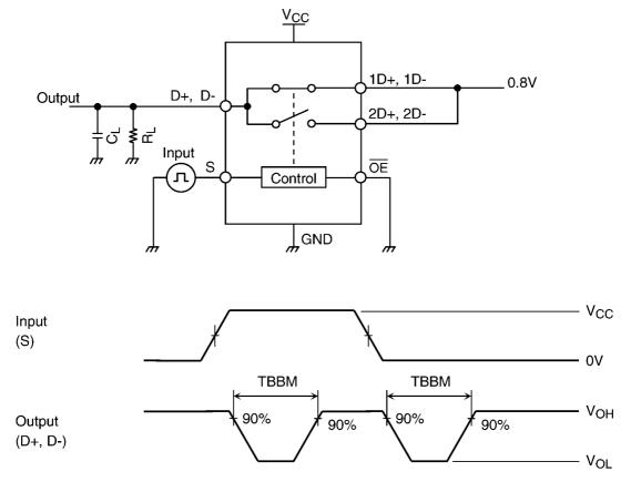
Fig. 11.3 Break Before Make (TBBM)
