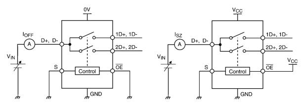
Fig. 11.10 Power-OFF Leakage Current
