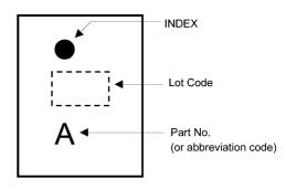
Fig. 5.2 UQFN10 (Top view)
