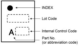
Fig. 5.1 UQFN10B (Top view)
