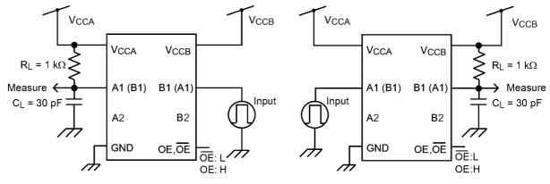
Fig. 13.1 t<sub>PLH</sub>, t<sub>PHL</sub> Test Circuits
