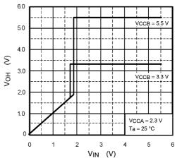
Fig. 14.3 Input/Output Characteristics (Typ.)  $V_{CCA}$  = 2.3 V, T<sub>a</sub> = 25 °C
