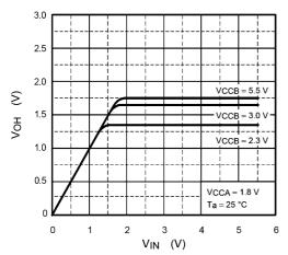
Fig. 15.2 Input/Output Characteristics (Typ.)  $V_{CCA}$  = 1.8 V, T<sub>a</sub> = 25 °C
