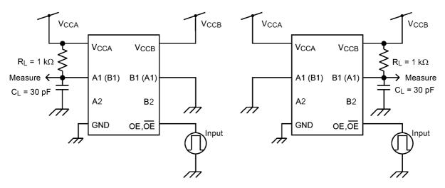
Fig. 13.2 t<sub>PLZ</sub>, t<sub>PZL</sub> Test Circuits
