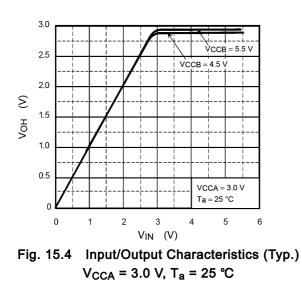
Note: The above characteristics curves are presented for reference only and not guaranteed by production test, unless otherwise noted.
