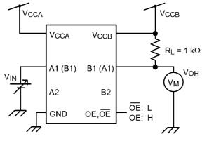
Fig. 14.1 Test Circuit
