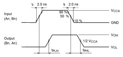
Fig. 13.3 AC Waveform of tPLH, tPHL
