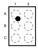
A1: VOUT B1: VOUT C1: GND A2: VIN B2: VIN C2: CONTROL
