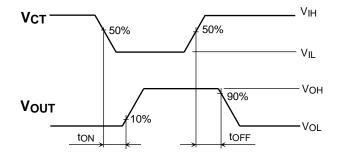
Figure 1 t<sub>r</sub>, t<sub>f</sub>, t<sub>ON</sub>, t<sub>OFF</sub> Waveforms
