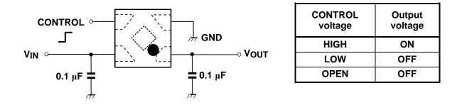
The figure above shows the example of configuration for using a Low-Dropout regulator. Insert a capacitor at VOUT and VIN pins for stable input/output operation. (Ceramic capacitors can be used.)
