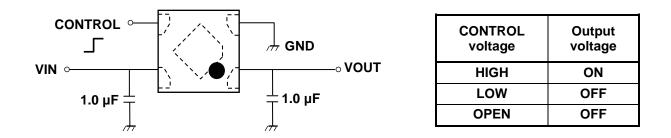
The figure above shows the recommended configuration for using a Low-Dropout regulator. Insert a capacitor at V<sub>OUT</sub> and V<sub>IN</sub> pins for stable input/output operation. (Ceramic capacitors can be used).
