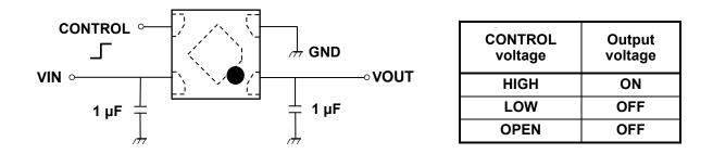
The figure above shows the recommended configuration for using a Low-Dropout regulator. Insert a capacitor at V<sub>OUT</sub> and V<sub>IN</sub> pins for stable input/output operation. (Ceramic capacitors can be used).
