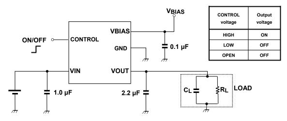
The figure above shows the Example of configuration for using a Low dropout regulator. Insert a capacitor at VIN, VOUT and VBIAS pins for stable input/output operation. (Ceramic capacitors can be used).
