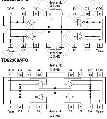
TD62308APG DIP16-P-300-2:54A TD62308AFG HSOP16-P-300-1.00
