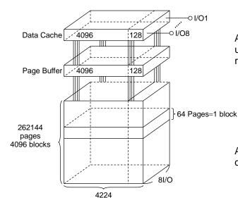
A page consists of 4224 bytes in which 4096 bytes are used for main memory storage and 128 bytes are for redundancy or for other uses.
