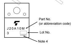
Note 4: A line under a Lot No. identifies the indication of product Labels Not underlined: [[Pb]]/INCLUDES > MCV Underlined: [[G]]/RoHS COMPATIBLE or [[G]]/RoHS [[Pb]]
