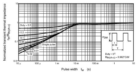
Fig. 8.13 r<sub>th</sub> - t<sub>w</sub> (Guaranteed Maximum)
