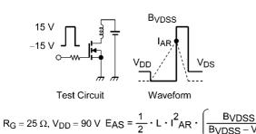
Fig. 8.16 Test Circuit/Waveform
