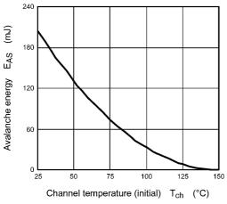
Fig. 8.14 E<sub>AS</sub> - T<sub>ch</sub> (Guaranteed Maximum)
