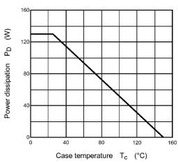
Fig. 8.15 P<sub>D</sub> - T<sub>c</sub> (Guaranteed Maximum)
