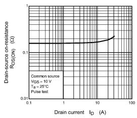
Fig. 8.6  $R_{DS(ON)}$  -  $I_D$
