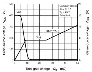
Fig. 8.12 Dynamic Input/Output Characteristics
