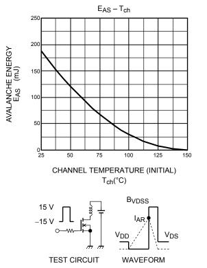
$$\begin{aligned} R_G &= 25~\Omega \\ V_{DD} &= 90~V,~L = 20.5~mH \end{aligned} \qquad E_{AS} &= \frac{1}{2} \cdot L \cdot I^2 \cdot \left( \frac{BVDSS}{BVDSS - VDD} \right) \end{aligned}$$
