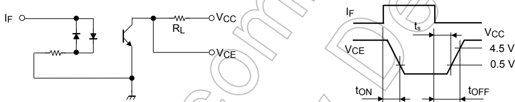
Fig. 1 Switching time test circuit
