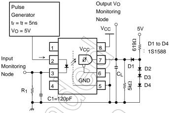
C<sub>1</sub> is peaking capacitor. The probe and jig capacitances are included in C<sub>1</sub>.
