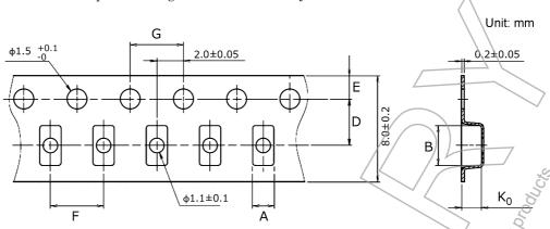
Table Tape Dimensions (unit: mm, tolerance: ±0.1)
