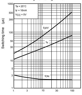
Load resistance  $\ R_L \ (k\Omega)$
