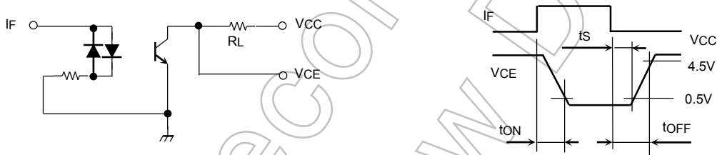
Fig. 1: Switching operating conditions
