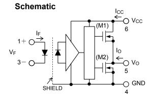
Note: A 0.1-μF bypass capacitor must be connected between pins 6 and 4.
