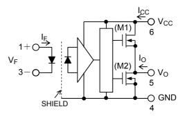
A  $0.1\mu F$  bypass capacitor must be connected between pins 6 and 4. (See Note 6.)
