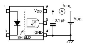
Fig. 12.3 IDDL Test Circuit
