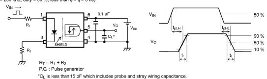
Fig. 12.5 Switching Time Test Circuit and Waveform
