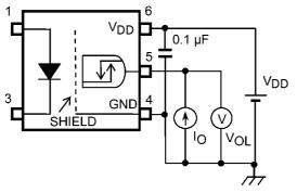
Fig. 12.1 V<sub>OL</sub> Test Circuit
