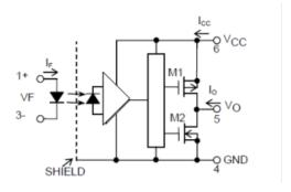
A ceramic capacitor (0.1  $\mu$ F) should be connected from pin 6 (VCC) to pin 4 (GND) to stabilize the operation of the high gain linear amplifier. Failure to provide the bypass may impair the switching property. The total lead length between capacitor and coupler should not exceed 1 cm.
