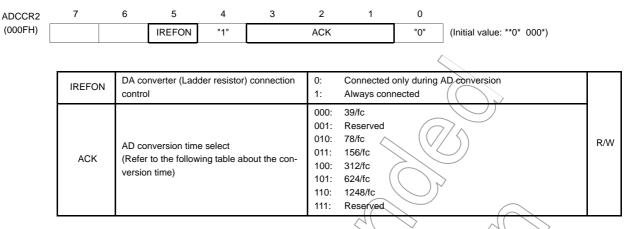
Note 1: Always set bit0 in ADCCR2 to "0" and set bit4 in ADCCR2 to "1".
