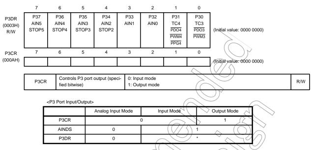
Note 1: When using the port for key-on wakeup input (STOP2 to 5), set the P3CR register's corresponding bits to 0.
