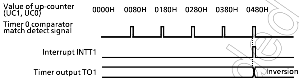
Figure 3.8 (11) Timer output by 16-bit timer mode
