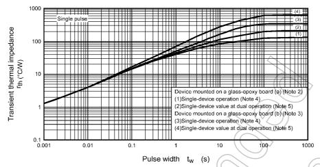
Fig. 8.1.12 r<sub>th</sub> - t<sub>w</sub> (Guaranteed Maximum)
