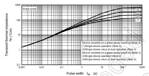
Fig. 8.2.12 r<sub>th</sub> - t<sub>w</sub> (Guaranteed Maximum)
