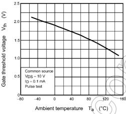
Fig. 8.2.9 V<sub>th</sub> - T<sub>a</sub>
