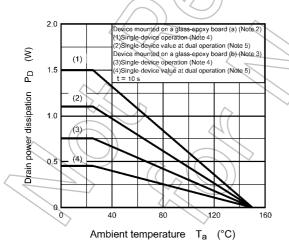
Fig. 8.2.11 P<sub>D</sub> - T<sub>a</sub> (Guaranteed Maximum)
