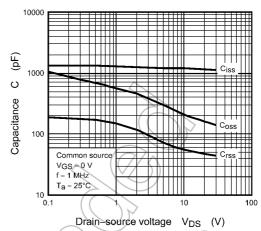
Fig. 8.2.8 Capacitance - VDS
