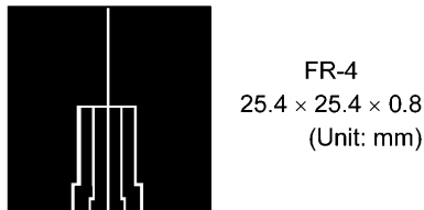
Fig. 5.1 Device Mounted on a Glass-Epoxy Board (a)
