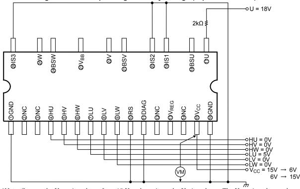
\*Note: Sweeps the V<sub>CC</sub> pin voltage from 15 V and monitors the U pin voltage. The V<sub>CC</sub> pin voltage when output is off defines the under-voltage protection operating voltage. Also sweeps from 6 V to increase. The V<sub>CC</sub> pin voltage when output is on defines the under voltage protection recovery voltage.
