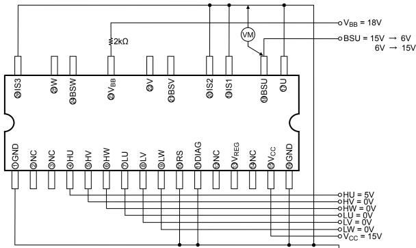
\*Note: Sweeps the BSU pin voltage from 15 V to decrease and monitors the VBB pin voltage. The BSU pin voltage when output is off defines the under voltage protection operating voltage. Also sweeps the BSU pin voltage from 6V to increase and change the HU pin voltage at  $5 \text{ V} \rightarrow 0 \text{ V} \rightarrow 5 \text{ V}$  each time. It repeats similarly output is on. When the BSU pin voltage when output is on defines the under voltage protection recovery voltage.
