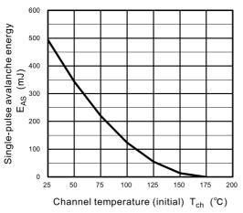
Fig. 8.15 E<sub>AS</sub> - T<sub>ch</sub>(Guaranteed Maximum)
