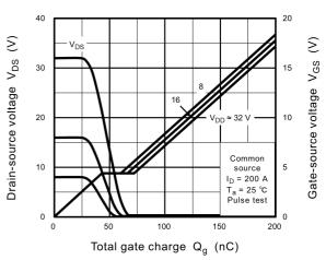
Fig. 8.14 Dynamic Input/Output Characteristics
