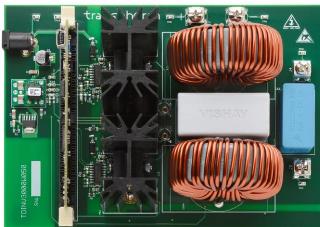
Figure 1. TDINV3000W050_0v4 inverter evaluation board
