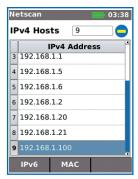
Display list of IP and MAC addresses of every device connected to the network.
